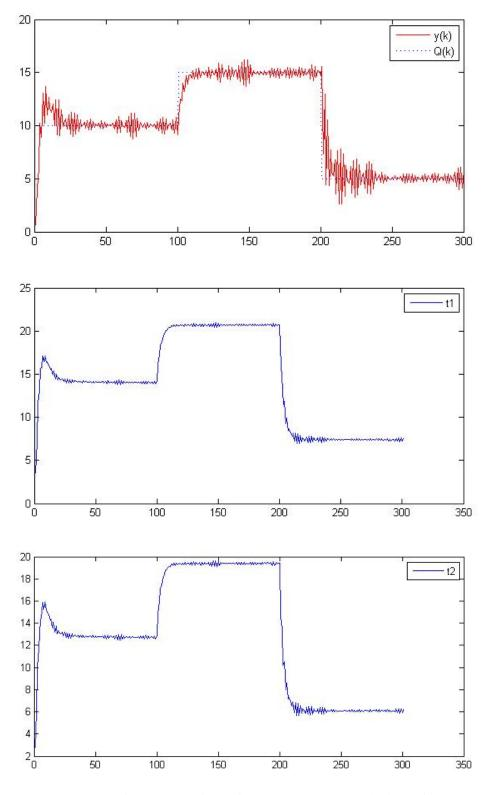
Figure 5 Tracking Performance of the Output and the Variation of Inputs with *W*=1.4 and *P*=I
