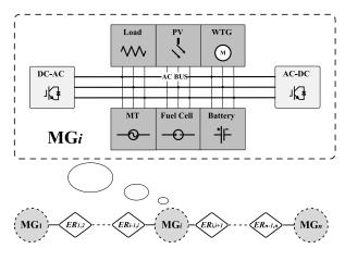
Figure 1. Series-Shaped Structure of EI.
