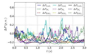
Figure 5. Power deviations of loads, PV units and WTGs.
