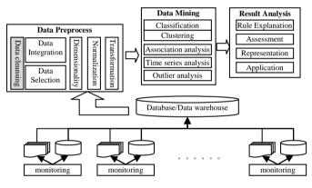
Fig. 1 Flowchart of advanced analysis for power quality
