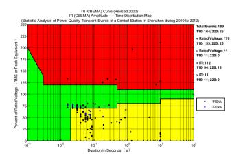
Fig. 8 Statistic results of monitoring data three of power quality after cleaning
