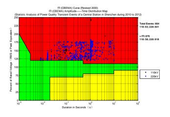
Fig. 5 Statistic results of monitoring data two of power quality before cleaning
