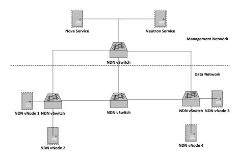
Fig. 4. Virtualized deployment of NDN
