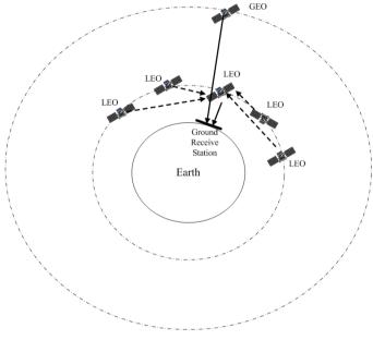
Fig.3 GEO and LEO hybrid satellite space energy network transmission (non-FOV ground receiving station)
