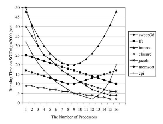
Fig. 6. Case study: applications. The timings shown in the figure are PACE performance prediction results for the execution of these applications on an SGI Origin2000.
