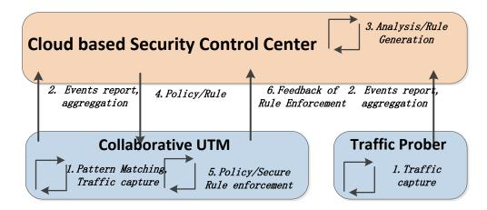
Figure 2. The work principle of Collaborative Network Security Management System with
