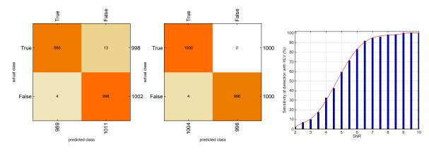
FIG. 4: Left panel: confusion matrix of a classifier on a test set with SNR = 8 (sensitivity is 98.70%). Middle panel: confusion matrix of a classifier on a test set with SNR = 9 (sensitivity is 100% for all signals with a higher SNR). Right panel: sensitivity of detection varying with the SNR, where, the false alarm rate = 0.4%.
