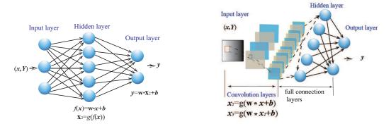
FIG. 3: Left panel: Traditional neural network (NN), in which the neurons (blue spheres) are connected to neurons in other layers by synapses (arrows). In the training process, the NN gets input  $\vec{x}$  and  $\vec{Y}$  and produces output  $\vec{y}$ . Right panel: Illustration of a DNN structure with convolution layers and fully connected layers, where \* is a convolution operator.
