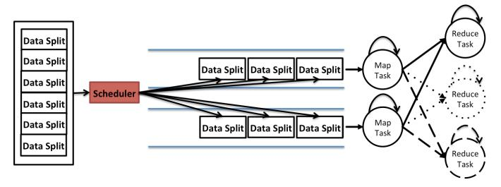
Figure 4(a). Initially six data splits arrive. Without knowing the compute capacity of each Map task, scheduler divides the workload evenly between the two queues, each one having three data splits.
