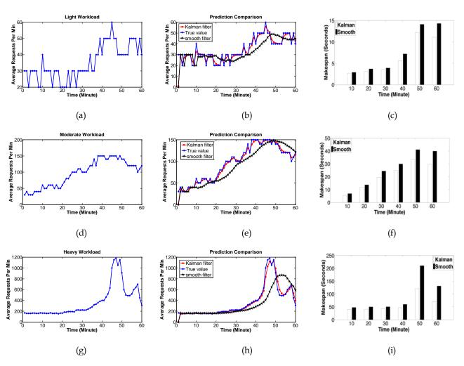
Figure 7. Comparison under three types of workloads. Figure (a)(d)(g) are light, moderate and heavy workload respectively;
