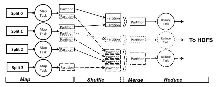
Figure 2. A MapReduce framework splits the input file into 4 segments, and each segment corresponds to one Map task.
