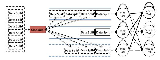
Figure 5. Demonstrates of adding an adaptive Map task. Continued from the previous example, if the input data split count is six, the scheduler adaptively launches one Map task instead of feeding all the data splits to the queues. The other three data splits are moved to the newly added Map task.
