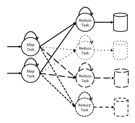
Figure 6. A graphical illustration shows one parallel Reduce task being added. This added Reduce task brings no benefit in the data shuffling stage but results to a reduced data volume to be processed/outputted for each Reduce task.
