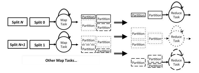
Figure 3. A demonstration of task-level adaptive MapReduce framework which processes streaming data. Each Map and Reduce task has a non-stop running daemon function which continuously processes the input data.
