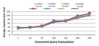
Fig. 7 Data query experiments in concurrent query transactions with our system.
